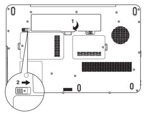
Figure 6-3 Securing the battery pack
